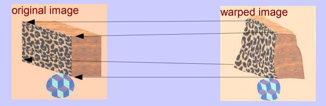
Warping needs a continuous function f(x,y) that is an interpolation of feature points
